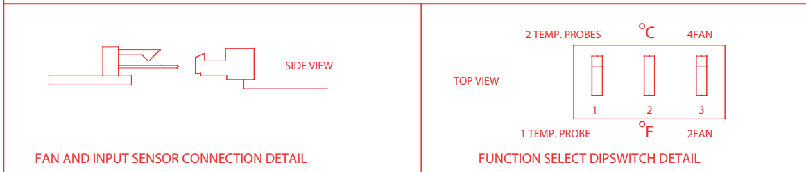
MAIN ISOBOX CONTROL BOARD CONNECTION DIAGRAM
